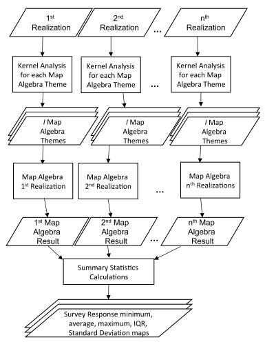
Figure 2: The stochastic simulation map algebra process.
